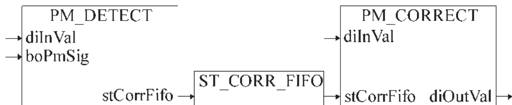
Fig. 11. Block diagram of a PMC
