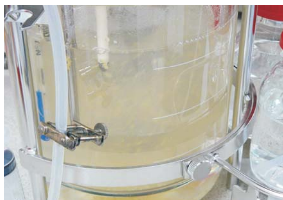
Fig. 2. Fed-batch cultivation of Linum tauricum suspension cultures in a 2 litre stirred tank bioreactor
