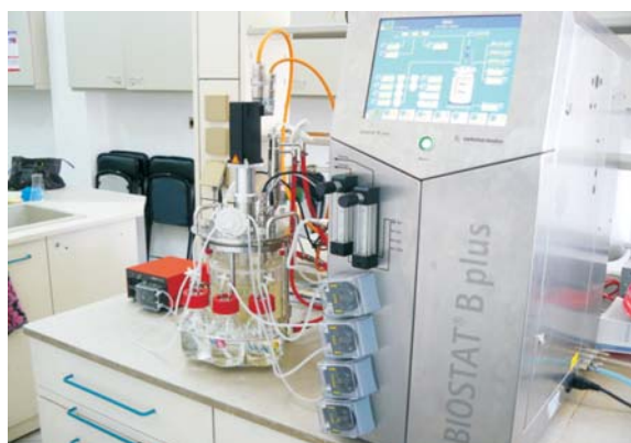
Fig. 2. Fed-batch cultivation of Linum tauricum suspension cultures in a 2 litre stirred tank bioreactor
