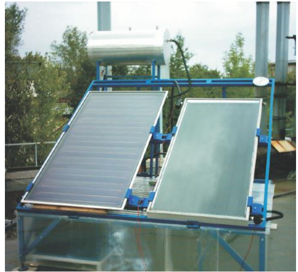
Fig. 2. General view of the solar collector test stand
