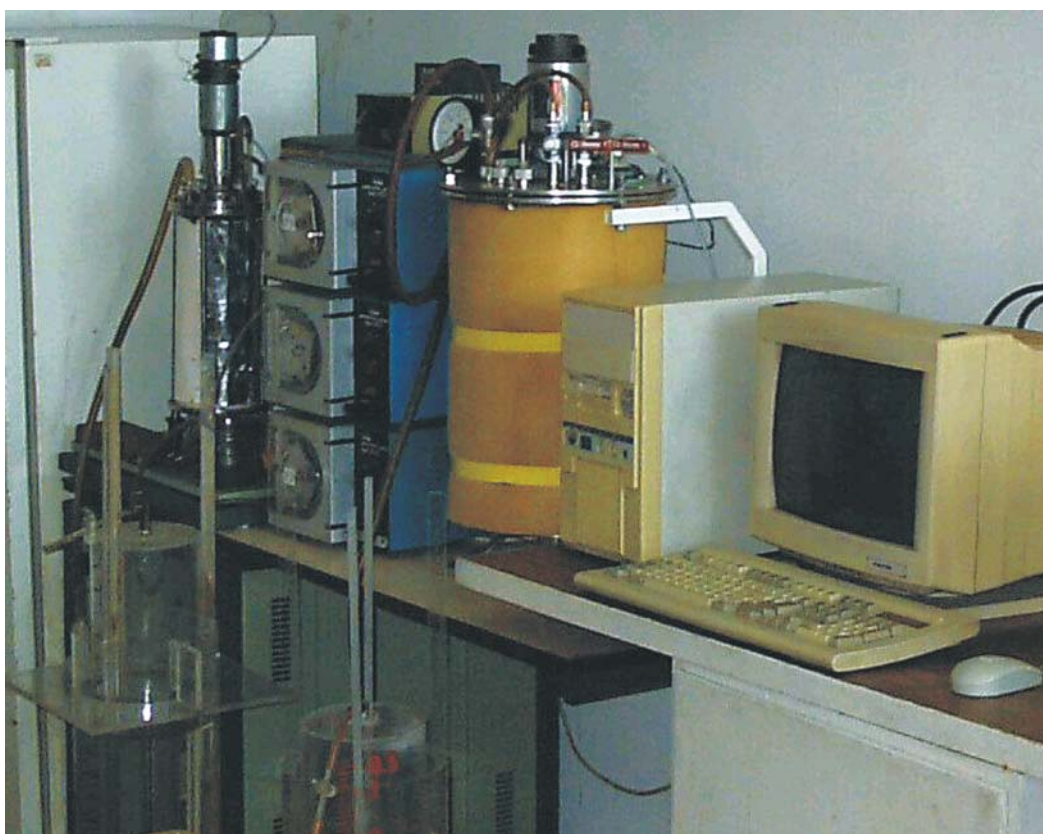
Fig. 2. Laboratory cascade of two anaerobic bioreactors
